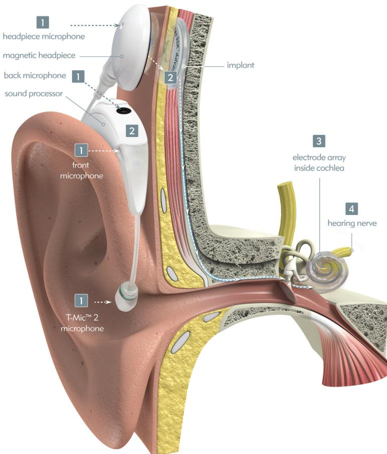
**Figure 3.** Schematic figure of a cochlear implant. The microphone captures the sound. The sound processor converts sound into signals. The magnetic headpiece transmits the signal to the implant. The electrode stimulates the acoustic nerve. Image courtesy of Advanced Bionics
